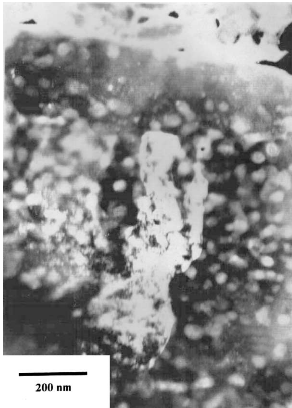
Fig. 3. Typical TEM micrograph of a PZT(53/47) film on Hastelloy substrate. In the micrograph the upper layer of a 5-fold sample is shown. The film exhibits closed porosity (bright dots) throughout the whole film thickness. Only the surface of each layer seems to be dense.
